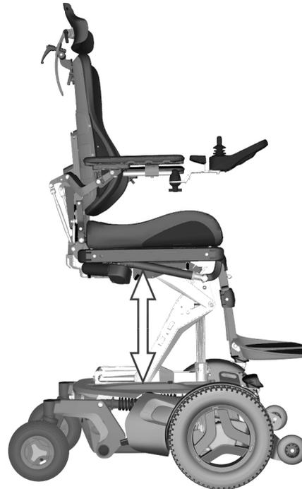
Figure 10. Electric Seat Lift
