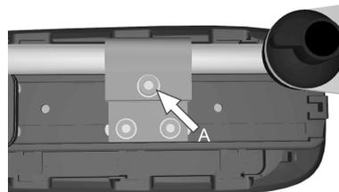
Figure 38. Length Adjustment screw (A)
