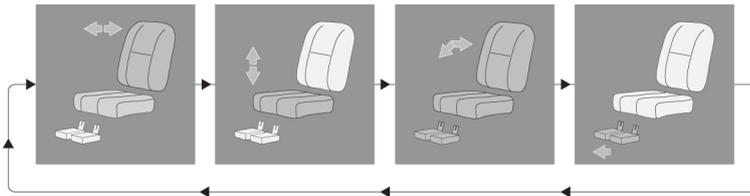
*Figure 66. Move the joystick to the left or right to select a function. The icon for the function selected appears in the display.*
