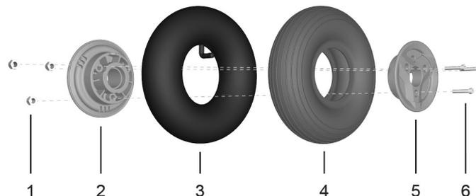
Figure 179. Inner tube replacement.
