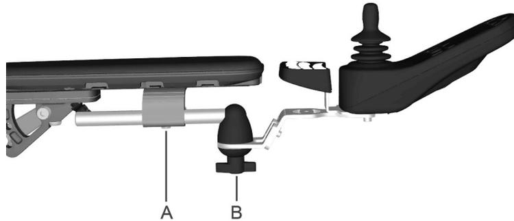
Figure 37. Length Adjustment screw (A) and Friction Joint Handle (B)
