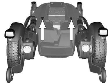
*Figure 181. The chassis covers are secured with two knobs.*
