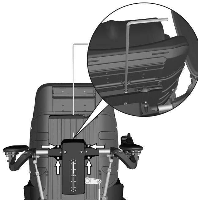
Figure 28. Adjusting the arm rest height
