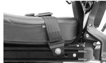
*Figure 21. Fitted Belt, left hand side.*
