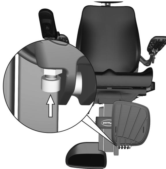
*Figure 25. The angle of the foot plates can be adjusted using a screw locked with a lock nut.*
