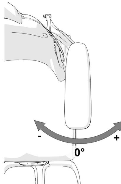
*Figure 26. The arm rest can be angled inwards/outwards.*
