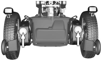
*Figure 3. Front Reflectors*
