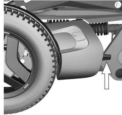
*Figure 169. Wheel lock engaged.*
