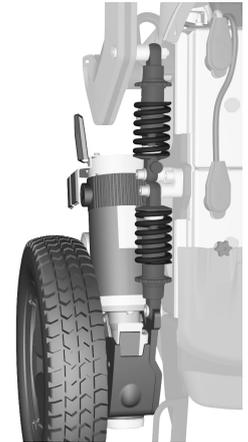
*Figure 2. Drive package and shock absorbers.*
