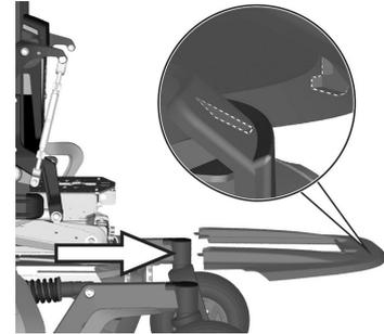
*Figure 182. The chassis top cover.*
