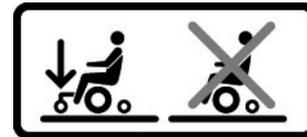
Figure 194. The support wheels must always be fitted when you drive.
