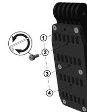
Figure 34. Height adjustment screw.
