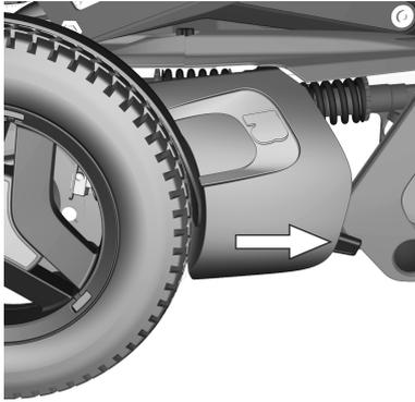
*Figure 167. Location of the release levers.*
