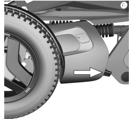
*Figure 175. Brake release lever*
