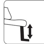
*Figure 153. Power Adjustable Leglength.*
