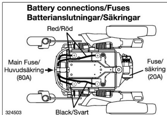
Figure 197. Battery Connections and Fuses.
