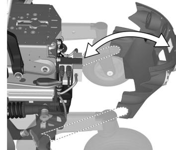
*Figure 183. The chassis rear cover.*
