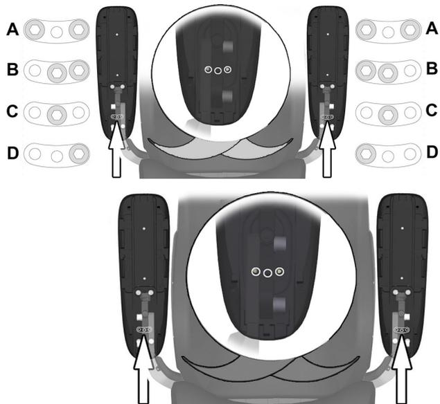
Figure 27. The endpoints are set by moving one or two screws between three different positions underneath the arm rest.
