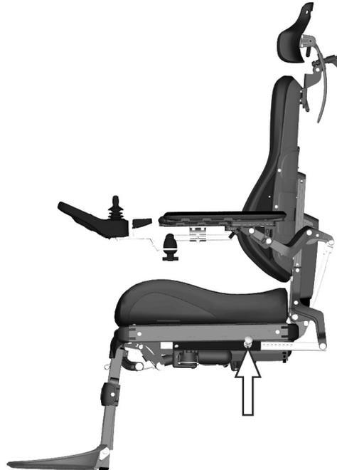
*Figure 16. Manual clamp Tube for the Backrest Recline*
