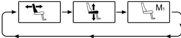
Figure 98. Move the joystick to the left or right to select a function. The icon for the function selected appears in the display.
