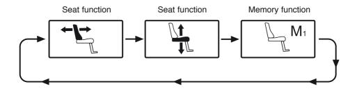
Move the joystick to the left or right to select a function. The icon for the function selected appears in the display.
