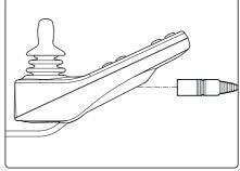
Charging Socket on the R-Net control panel.
