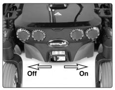
The circuit breaker is accessed through a hole in in the chassis cover.
