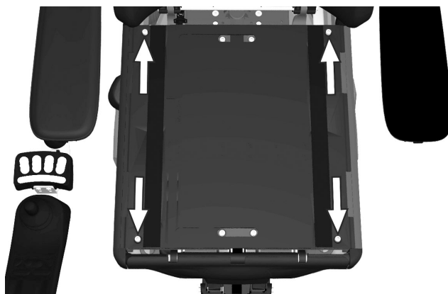
Figure 87. The seat plates are held in place by four screws.
