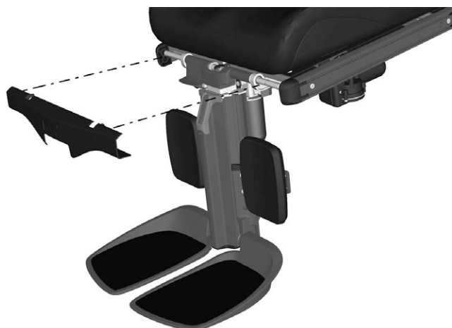
Figure 235. Mount the legrest's top cover by carefully pressing its bracket into place on the legrest's fixing screws/spacers.
