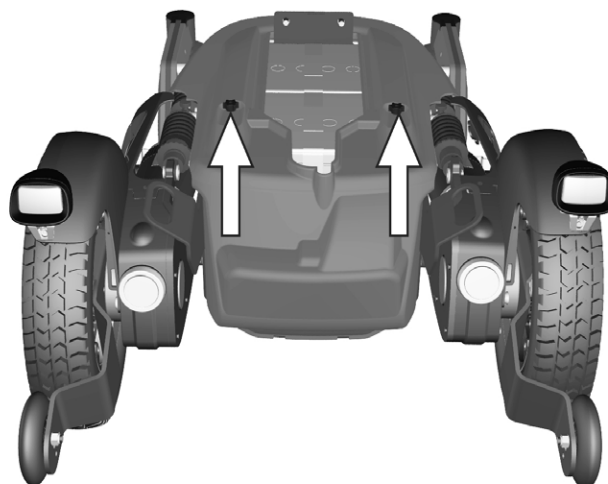
Figure 27. The chassis covers are secured with two knobs.
