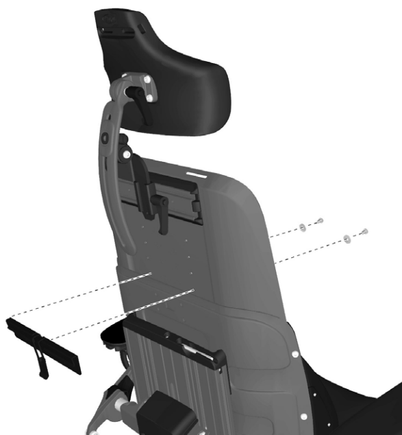
Figure 251. The locking mechanism is held in place by two screws.
