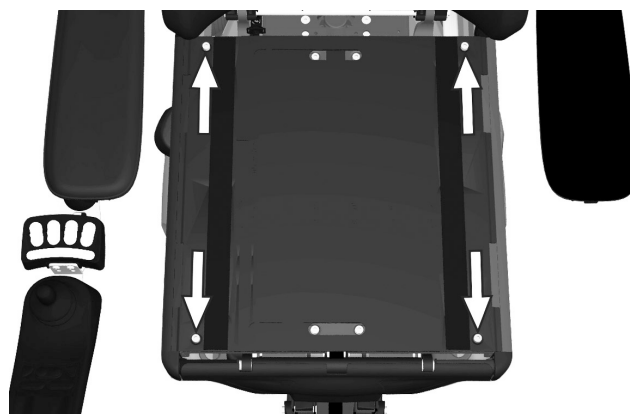
Figure 74. The seat plates are held in place by four screws.
