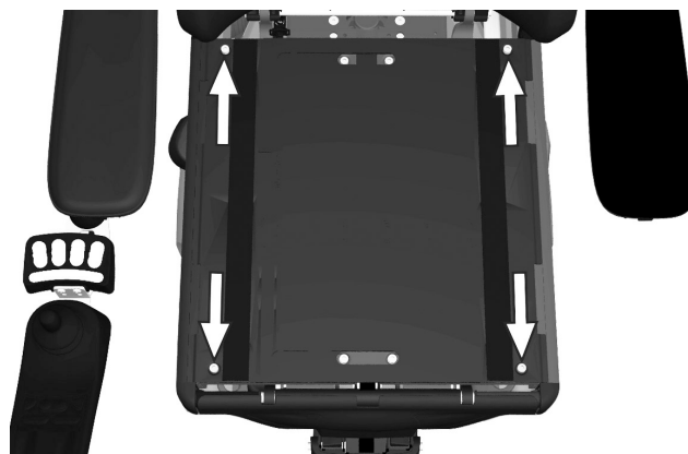
Figure 242. The seat plates are held in place by two screws at the back edge and two quick-mount clamps at the front.
