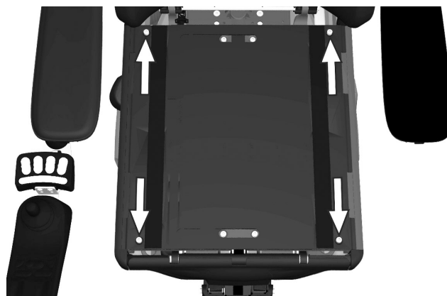
Figure 248. The seat plates are held in place by two screws at the back edge and two quick-assemble clamps at the front.
