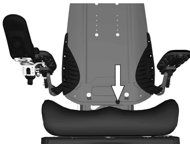
Figure 189. The lower backrest plate is secured by means of a knob.
