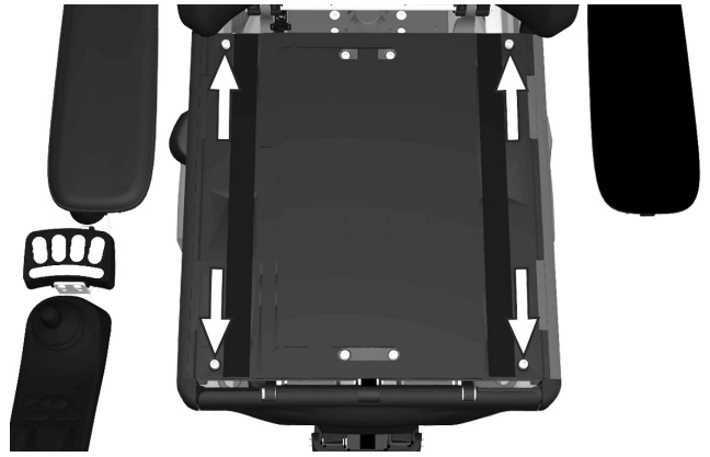
Figure 185. The seat plates are held in place by four screws.
