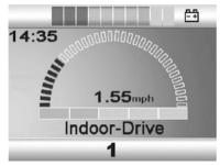
Figure 99. Standard display image with speed indicator.
