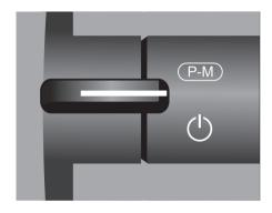
Figure 105. Power/Mode/Profile Paddle Switch.
