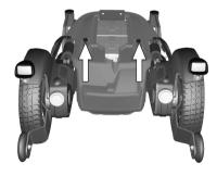
Figure 181. The chassis covers are secured with two knobs.
