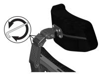
Figure 35. Adjust height / depth.
