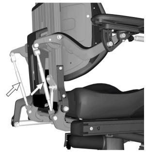
Figure 29. The position of the adjustment bars are secured with two nuts.
