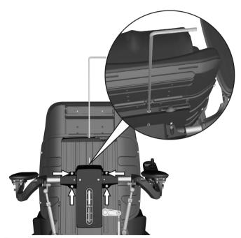
Figure 28. Adjusting the arm rest height
