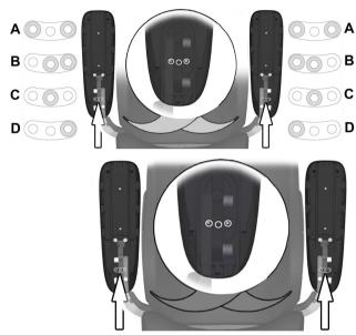
Figure 27. The endpoints are set by moving one or two screws between three different positions underneath the arm rest.
