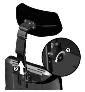
Figure 33. Removal of headrest.
