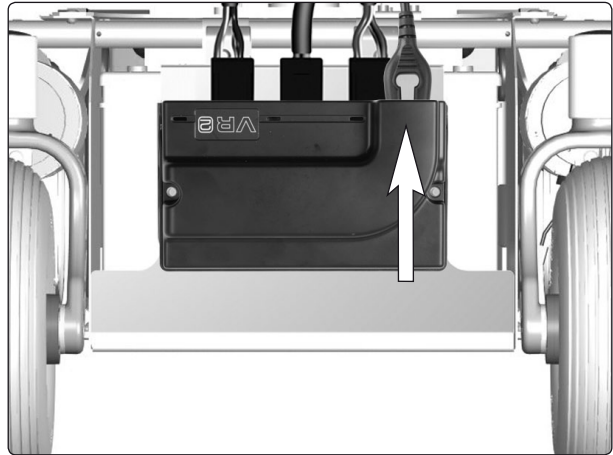
The control panel cabling is connected to the output stage.
