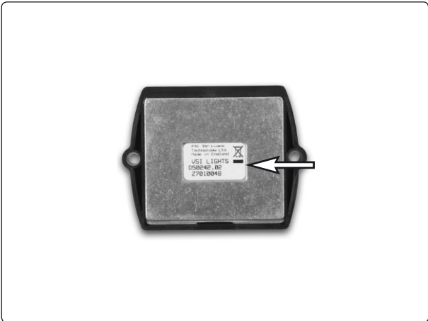
Control panel VR2 ID number
