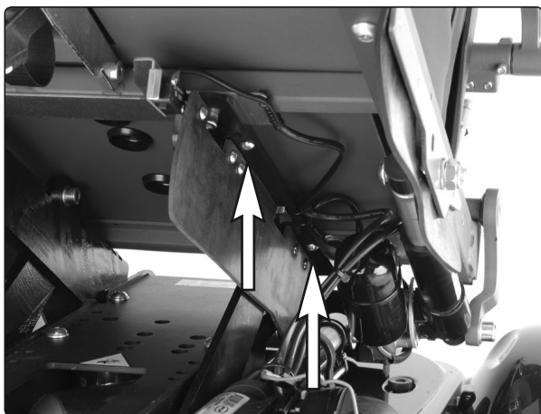
The crush protection devices on the left and right sides are held in place with two screws.
