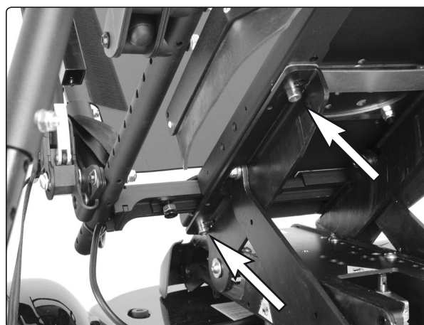
The seat is held in place with two screws on the left and right sides.
