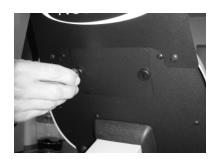
Use coin to remove battery access panel.
